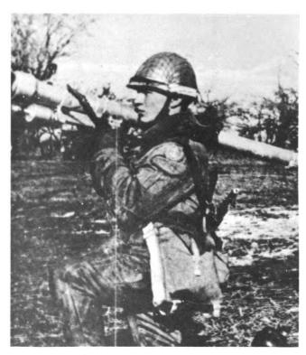
Figure 6-42 SA-7 GRAIL. The GRAIL is a shoulder-fired low-altitude surface-to-air missile, similar to the US Redeye, with a passive infrared guidance system. Shown above is a Polish marine demonstrating firing position.
